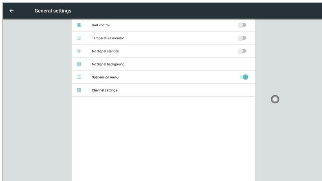
(1) Centralized control switch: The centralized control function is to remotely control some basic functions such as sound addition and subtraction and channel switching through the R232 serial port. To use the centralized control function, the centralized control switch needs to be turned on.
