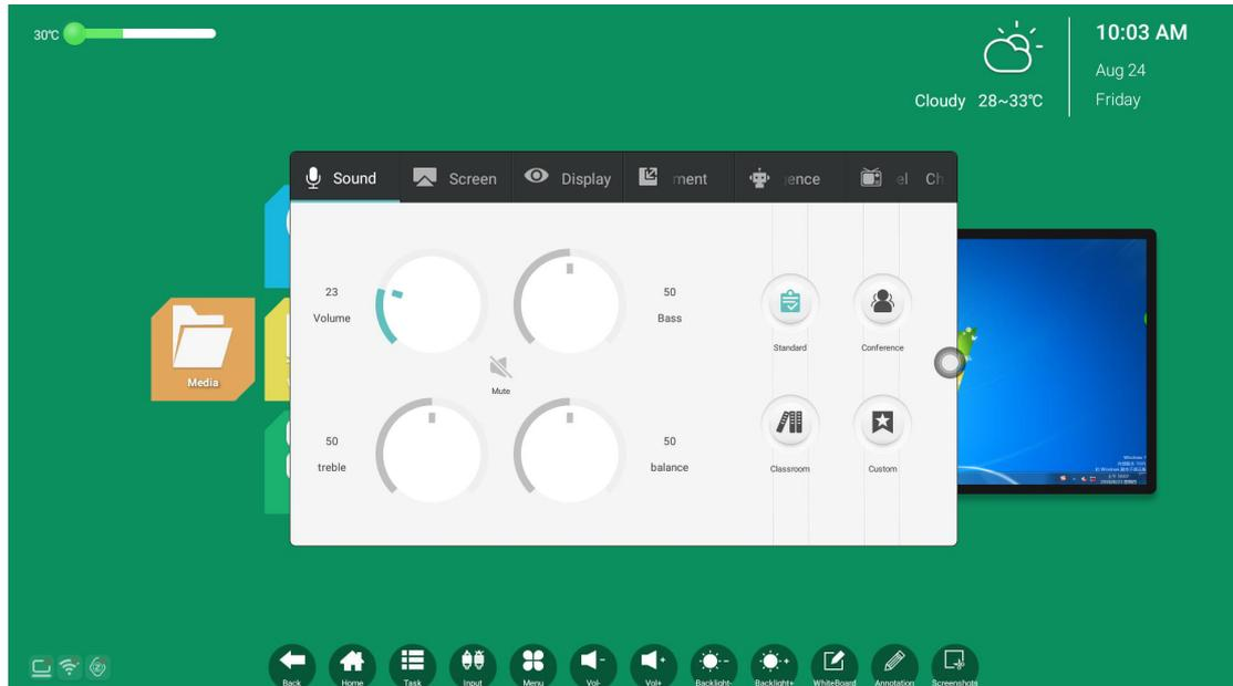
The system menu settings mainly include sound, screen, display, adjustment, smart, and channel function settings.
