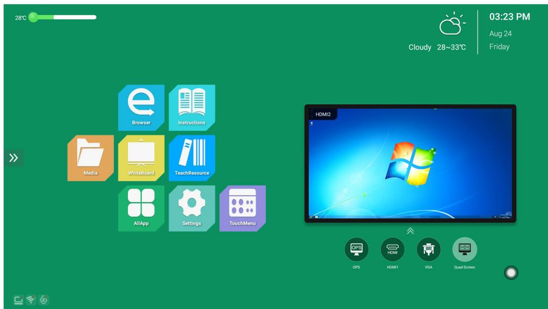
1. Quad screen: After the quad screen function is turned on, the preview screen of the Android home page will display a preview screen of four channels.
